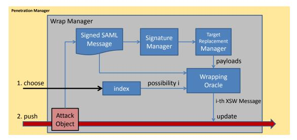
FIGURE 4.5: Wrapping Oracle Integration (based on Figure 28 in [10, page 55])
