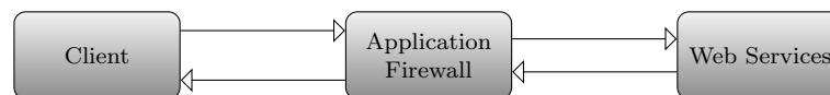
Figure 4: Security via SSL/TLS. A client wants to execute a web service operation which is protected by an application firewall.
