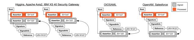
Figure 8: XML tree-based illustration of refined XSW attacks found in Type 1 signature applications.
