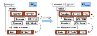
Figure 15: Unique identification of signed data applied on a SOAP message including two signed elements: The  $RP_{sig}$  module uniquely identifies the signed elements with a random value r and forwards this information along with the whole XML message.
