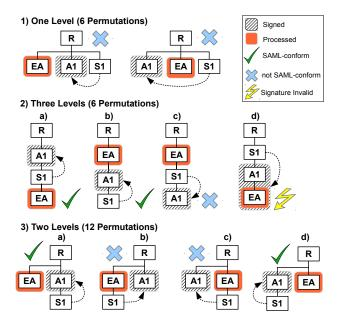
Figure 7: Possible variants for XSW attacks applied on messages with one signed SAML assertion divided according to the insertion depth of the evil assertion *EA*, the original assertion *A1* and the signature *S1*. The various permutations are labeled according to their validity and SAML-conformance.
